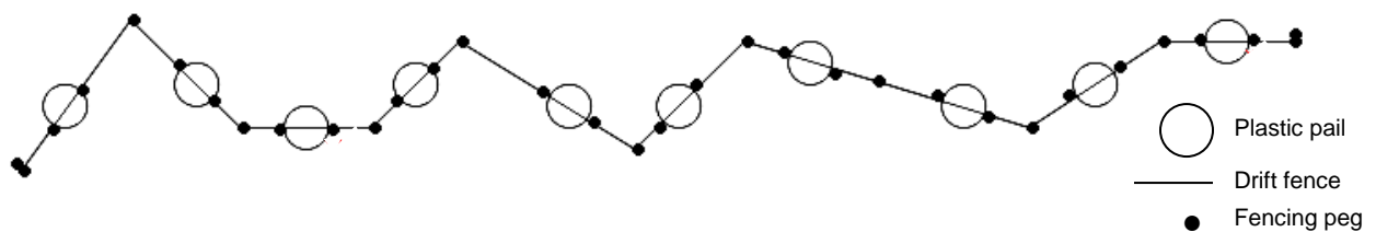
Figure 2. Diagram showing the structure of a constructed pitfall line (aerial view) including positions of buckets, pegs and flywire.
